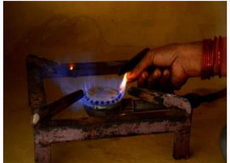
**Fig. 7 Fueling the biogas stove**
